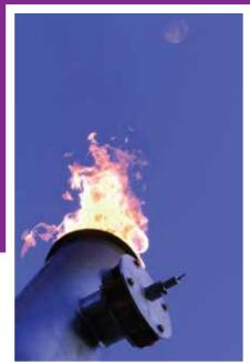
CESB — BKE flaring system are designed with priority to meet safety requirements and CDM specifications. Thermal heat, flue gas dispersion, noise level and visible smoke are important criteria to ensure plant operators and equipment are not exposing to hazardous zone.
